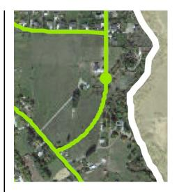
1. The master plan alignment runs directly through a FEMA Flood Zone. To construct a road through this property could require significant costs because there could be a need to bring in fill dirt, and it is possible that there could be environmental issues that might need to be mitigated or permitted.
